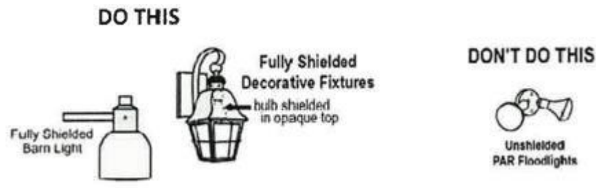
Examples of Fixtures
