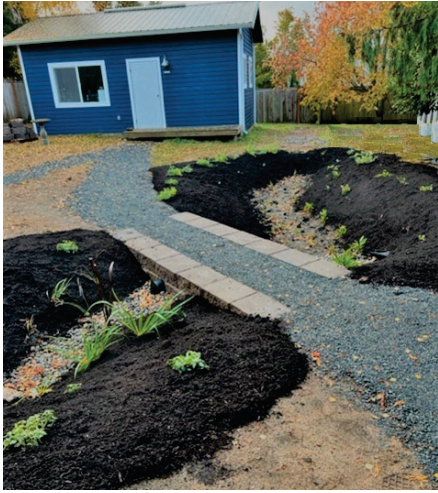
Rain Garden in Richmond Beach neighborhood soaks up rainwater from over 1,981 square feet of rooftop!
