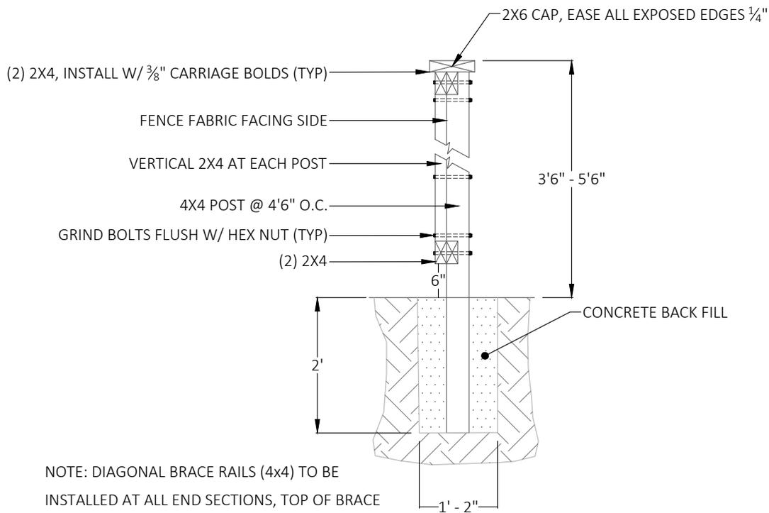
NOTE: DIAGONAL BRACE RAILS (4x4) TO BE INSTALLED AT ALL END SECTIONS, TOP OF BRACE AT TOP OF END SECTION/CORNER.
