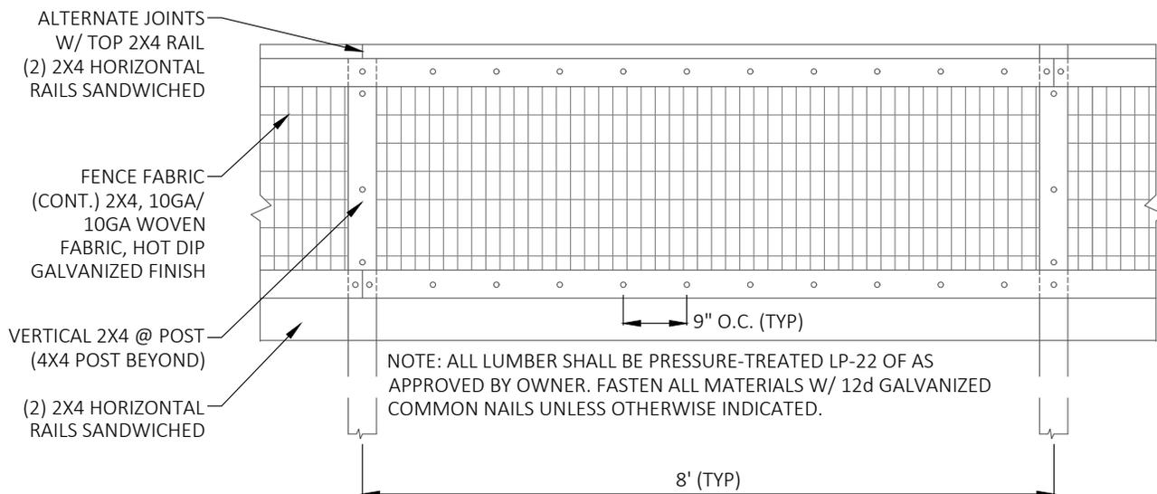
NOTE: ALL LUMBER SHALL BE PRESSURE-TREATED LP-22 OF AS APPROVED BY OWNER. FASTEN ALL MATERIALS W/ 12d GALVANIZED COMMON NAILS UNLESS OTHERWISE INDICATED.
