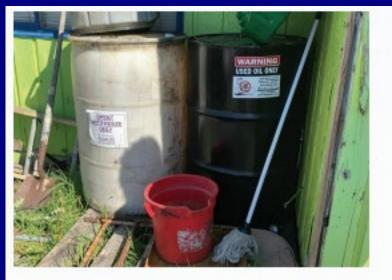
Before: Without secondary containment, any oil spilled during adding/removing materials from the drums would spill to the ground, causing soil contamination.
