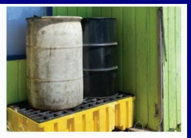
After: With secondary containment, even if there is a spill or overflow, any spilled materials will be captured with the secondary containment pallet and can be properly managed.
