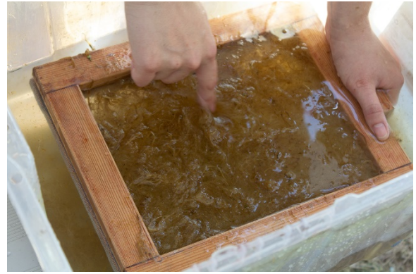
The fibers have reached maximum separation after being thoroughly beaten, and now disperse evenly in water.
