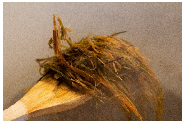
Scotch broom fibers after being separated from woody stem and being boiled in a solution of water and lye. The heat and alkalinity of the lye work to break down the chemical bonds holding individual fibers together.
