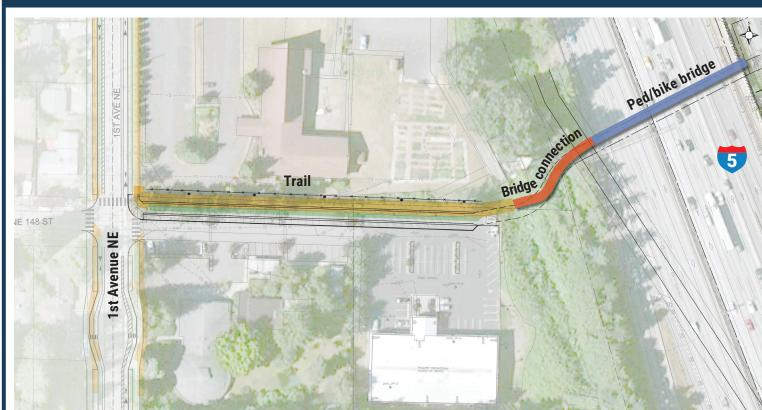
**FULL BUILD-OUT:** This portion will connect the bridge to 1st Avenue NE via a 16-foot shared path and planted buffer. The exact alignment is still being determined and the City is looking for ways to minimize impacts to trees and parking. The City is working closely with neighboring property owners as the design is refined.
