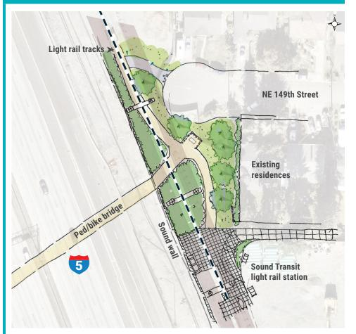
**DIRECT RAMP:** The ramp on the east side of the project will provide direct access to the future Shoreline South/148th Station, bus routes, and the future Trail Along the Rail. The direct ramp design will eliminate the need for stairs, providing easy access for travelers, on foot, on bicycle or using assisted modes of travel such as wheelchairs.
