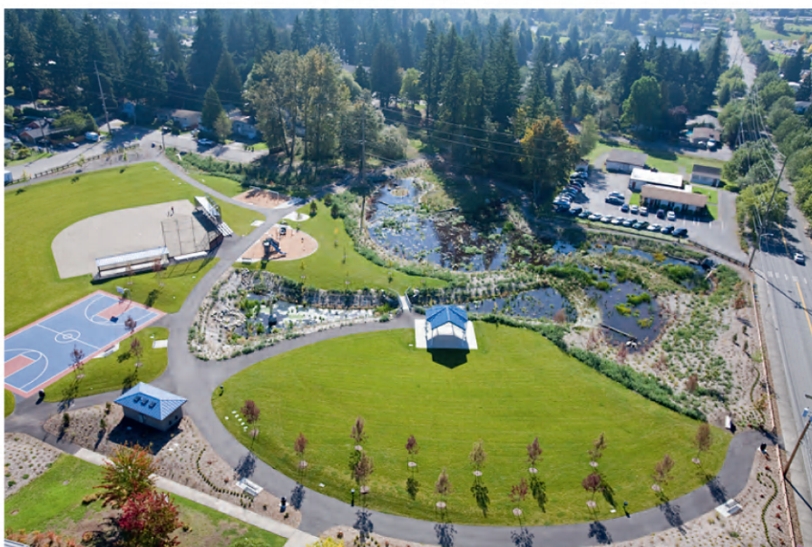
PHOTO: The detention pond at Cromwell Park manages stormwater naturally, using wetland habitat to store and filter runoff from the surrounding neighborhood.
