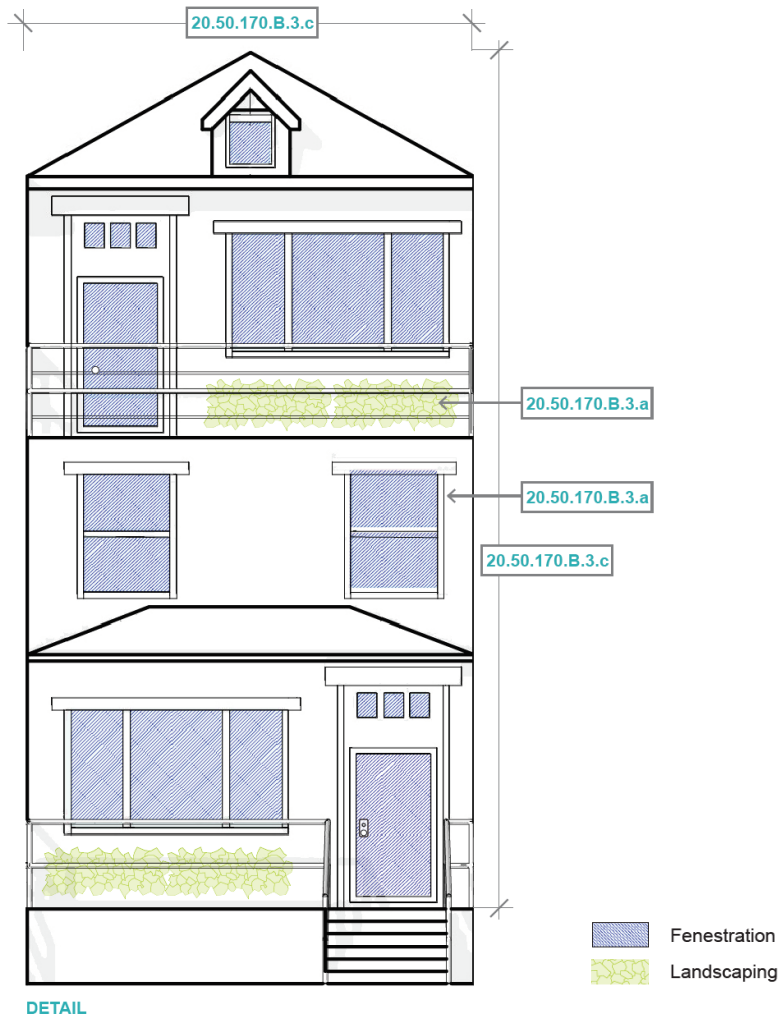
Building Modulation, Massing and Articulation Illustration 3: Illustration of No Blank Façade. The façade facing the right-of-way measures 650 square feet. The façade depicted has 235 square feet of fenestration and landscaping, which is 36 percent of the façade, meeting the requirement.
