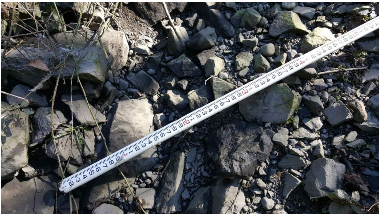
Photo 4. Typical riprap gradation within the entrenched channel reach, near the middle of the project area.
