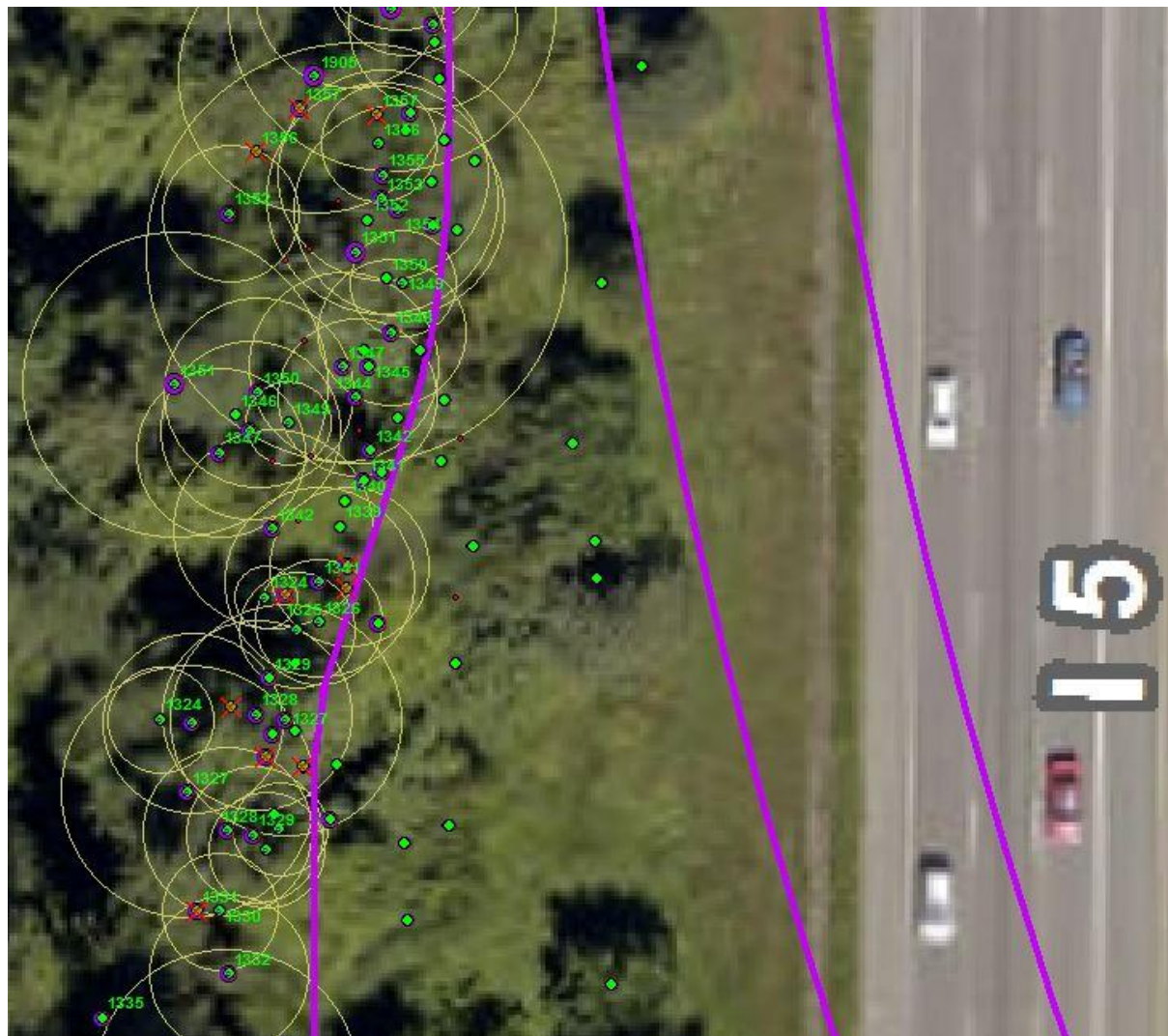
Figure 5. Tree Point Display on Aerial. Trees were documented over the entire Lynnwood Link LRT route. All of the documented information on each tree is available and retrievable through an internet based GIS Application for querying and displaying data and in an Excel spreadsheet within this application. This Figure is an example of how tree points, tag ID numbers and critical root zones are illustrated on the web based application for retrieval. The diameter of the circle is shown in relationship to the trunk diameter of the tree.
