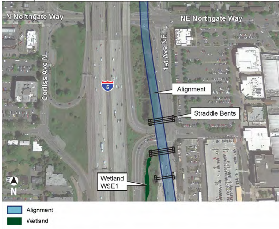
Figure 4-1 (D1) Minor Track Realignment at Northgate
