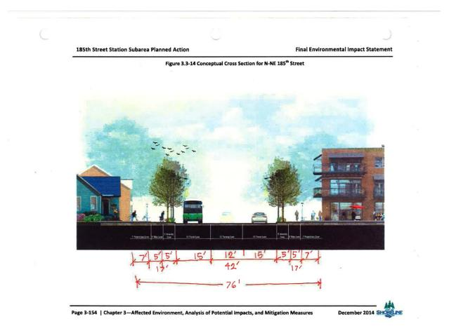
The above conceptual cross section for motorized travel does fit the 185<sup>th</sup> Street roadway improvements within the current Master Street Plan's *curb-to-curb* width of 42'. However, it exceeds the Master Street Plan's overall 66' *cross-section* which includes non-motorized improvements by 10'. The extra 10' is proposed in an effort to achieve "Transit-Oriented Community" goals and policies, which encourage mixed-use
