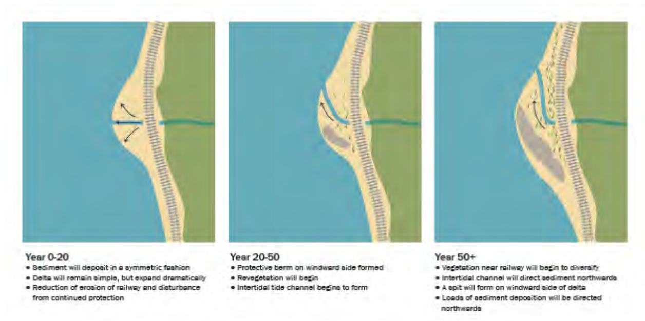
Figure 8. Diagram Illustrating Expected Progression of Delta Formation at the Mouth of Boeing Creek.
