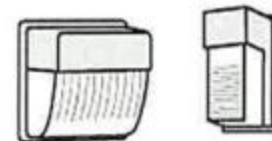
Unshielded Wallpacks & Unshielded or Poorly-shielded Wall Mount Fixtures
