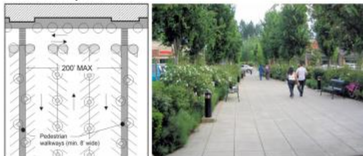
Parking Lot Walkway
