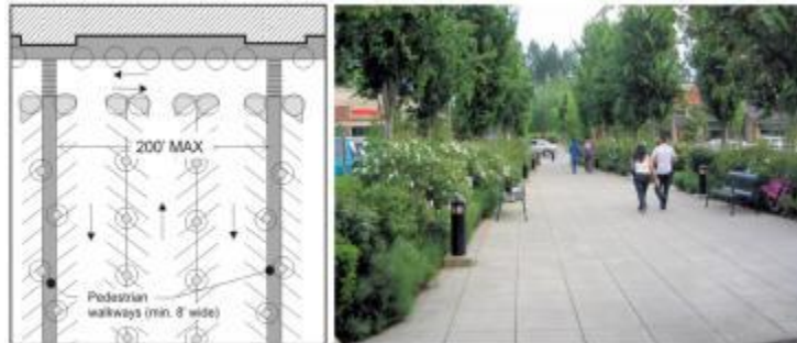
Parking Lot Walkway
