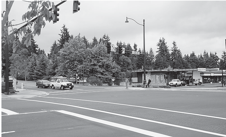
The crosswalks in the North City area have a distinct pattern and color to make them more visible to enhance safety.
