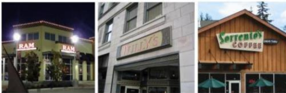
Individual backlit letters (left image), opaque signs where only the light shines through the copy (center image), and neon signs (right image).
