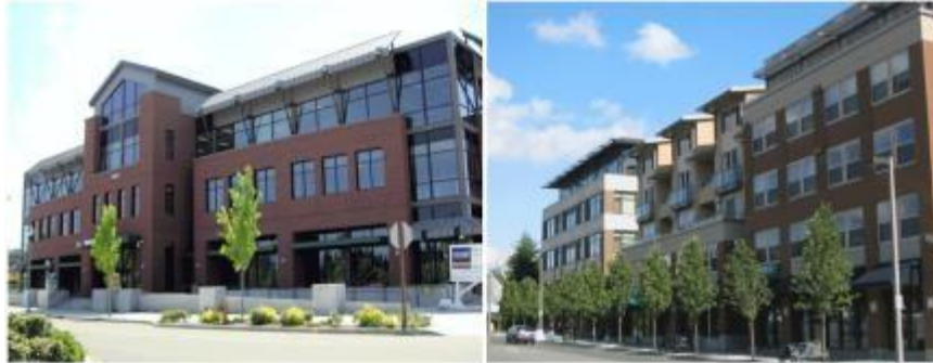
Facade Widths Using a Combination of Facade Modulation, Articulation, and Window Design
