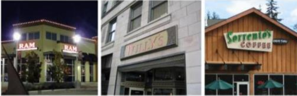
Individual backlit letters (left image), opaque signs where only the light shines through the copy (center image), and neon signs (right image).
