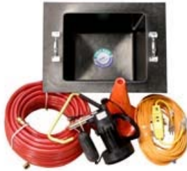
Figure 2. Various supplies used to collect pressure wash water and pump it to sewer.
