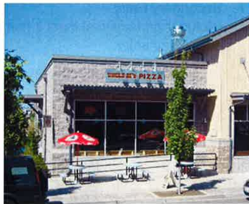
The left image uses smooth gray blocks on the vertical columns and beige split-faced blocks above the awnings. The storefront in the right image uses gray split face and some lighter, square, smooth-faced blocks below the storefront windows.
