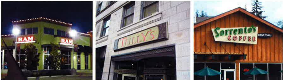
Individual backlit letters (left image), opaque signs where only the light shines through the letters (center image), and neon signs (right image).
