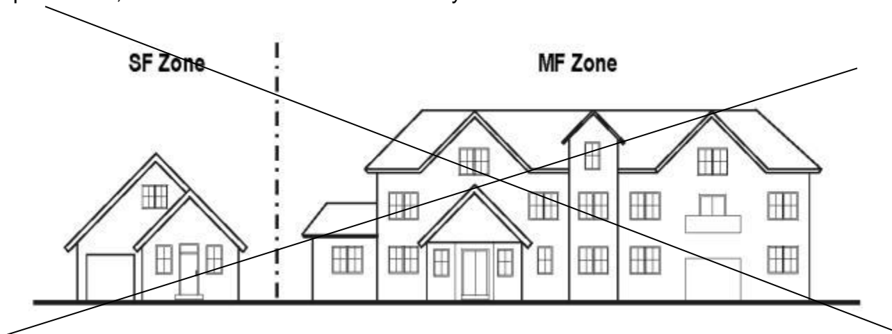
Figure 20.50.180(C): Stepping repeating elements such as entry porches help large buildings fit better with adjacent single-family neighborhoods.
