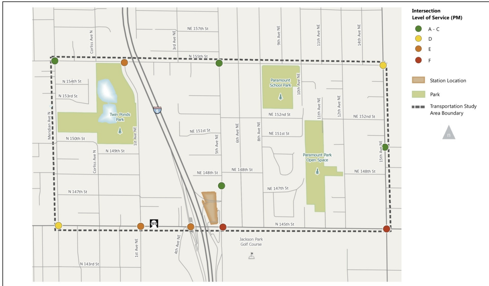
Figure 3.3-10 Intersection Level of Service (Alternative 1—No Action)
