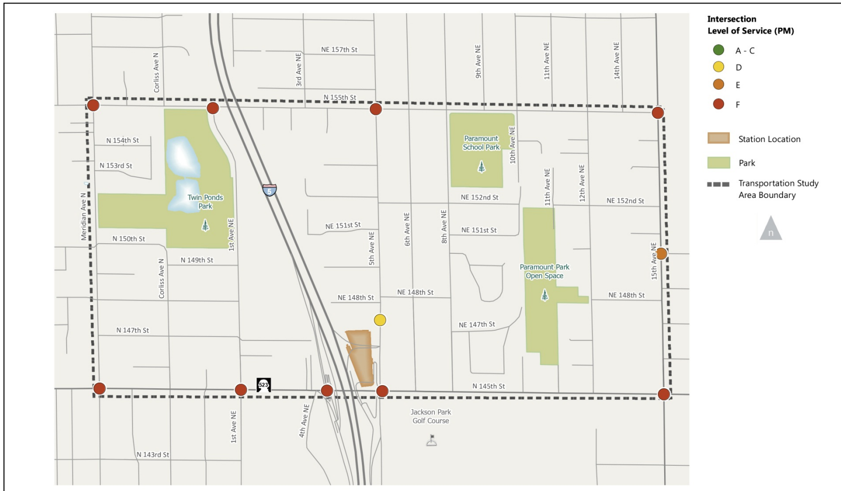
Figure 3.3-14. Intersection Level of Service for Alternative 3—Compact Community (Full Build-out)
