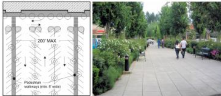
Parking Lot Walkway
